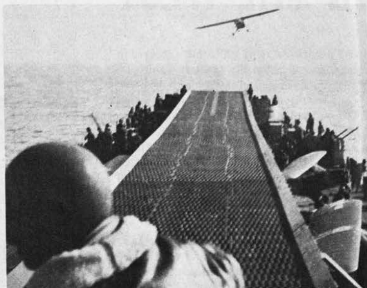
Coast-Guard-manned type at Anzio was fitted to land planes. Ships were converted on the spot and are not planned as long-time measures.
